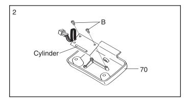
3. Connect the Wire (C) on the receiver to the wire extending from the Console Assembly (A). Make sure that no wires are pinched. Reattach the Pulse Receiver Cover (70) to the Console Assembly with the two 3/4" Screws (4). Discard the other wires included with the receiver.
